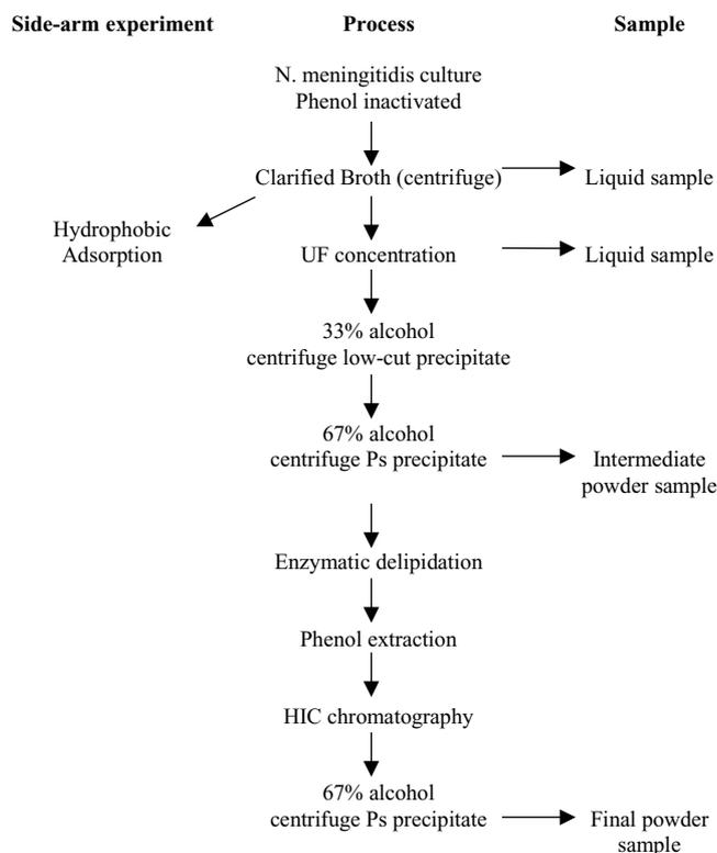
Fig. 1. MnPs purification flow diagram.
